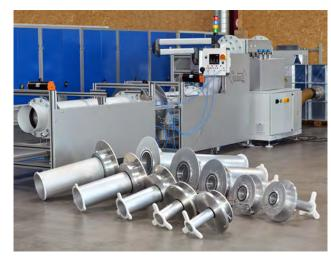
Rapid clamping system by the turret design for maximum 5 different nominal diameter up to DN150
