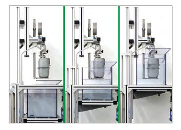
different pressures and the optional connection to detect the leakage rate makes the test rig universally applicable. The test rig is equipped with adaptors to connect different versions of gas meters. For an easy handling and a fast operation all necessary displays and operating instruments are installed in front of the operator.
